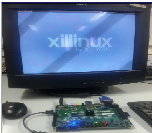
Figure 3. Booting of Xilinx from SD card.
