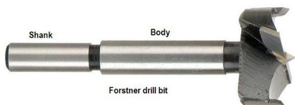
Figure 1. Forstner drill bit used for experimentation.
