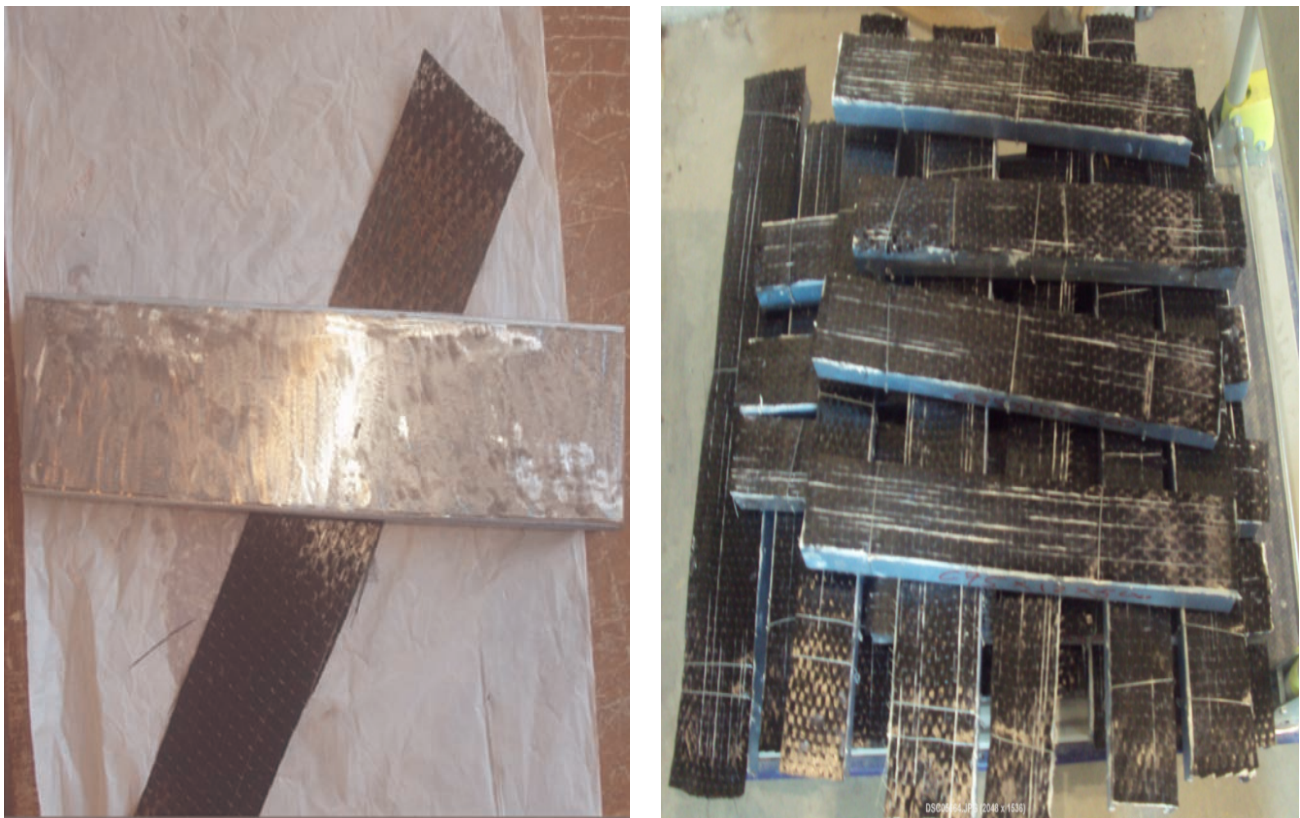
Figure 2. (a) Surface preparation (b) Prepared test specimens.
