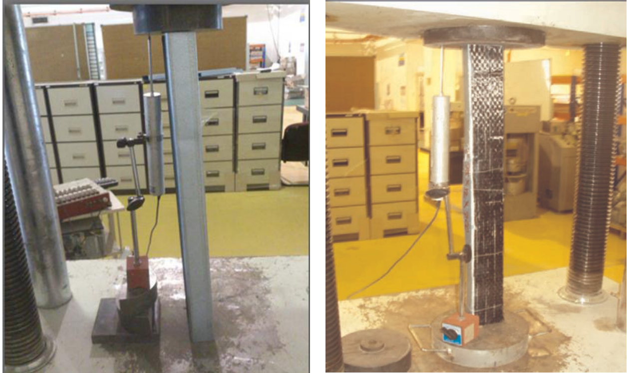
Figure 1. Test set up (a) plain cold formed steel (b) CFRP Strengthened cold formed steel.
