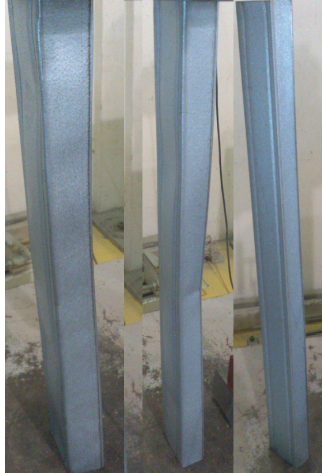
Figure 2. Failure modes shapes.
