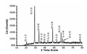
Figure 3. The XRD pattern of the no-calcined Dy<sub>2</sub>O<sub>3</sub> (Sample 1) nanoparticle, cubic structure, without additional phase.
