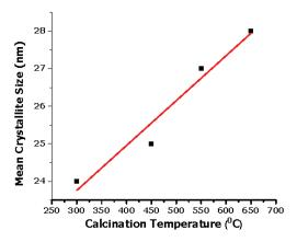
Figure 5. Variation of mean crystallite size against calcination temperature. The first point is for no-calcined sample and the temperature is the furnace temperature.
