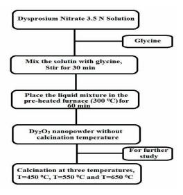
Figure 1. Flow chart of Dy<sub>2</sub>O<sub>3</sub> nanoparticles preparation by combustion process.
