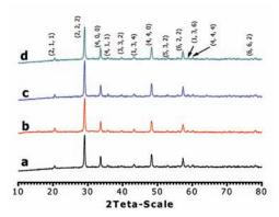
Figure 4. The XRD patterns of a) no-calcined sample b) calcined sample at T=450°C, c) calcined sample at T= 550°C, d) calcined sample at T=650°C.
