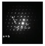
Figure 7. TEM diffraction pattern of no-calcined Dy<sub>2</sub>O<sub>3</sub> nanoparticles.
