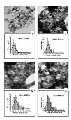
Figure 6. TEM images of Dy<sub>2</sub>O<sub>3</sub> prepared a) without calcination temperature, b) at 450°C calcination temperature, c) at 550°C calcination temperature, d) at 650°C calcination temperature.
