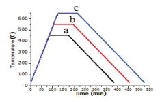
**Figure 2.** Calcination diagram of, a) sample 2, calcined at 450°C, b) sample 3, calcined at 550°C, c) sample 4, calcined at 650°C.
