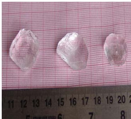
Fig. 1. Photograph showing the pure and proline added TGS crystals grown (from left: pure TGS, 5 & 10 wt% proline added)
