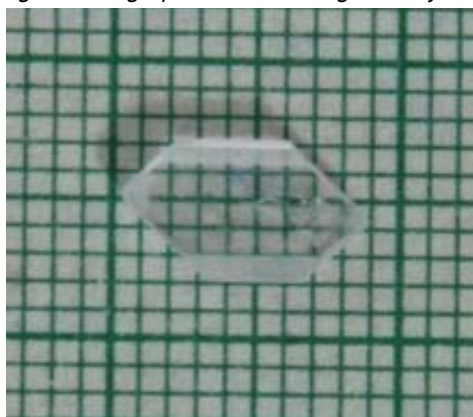
Fig. 1. Photograph of the CMBA grown crystal
