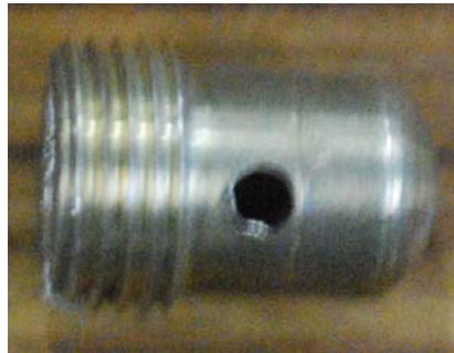
Plate 2. Swirl chamber of air assisted pressure swirl atomizer.
