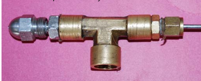
Plate 4. Complete assembly of air assisted atomizer.
