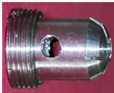
Plate 2. Swirl chamber of air assisted pressure swirl atomizer.
