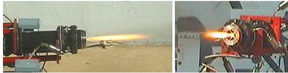
Fig.11. Static test of HTPB and RFNA
