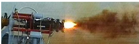
Fig.5. Test-01 of HTPB with 10%AP and RFNA
