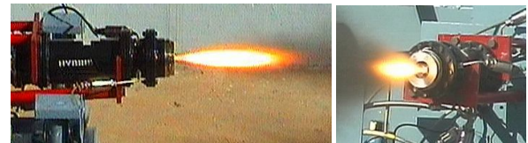
Fig.14. Static test of HTPB with 10%AP and RFNA
