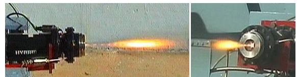
Fig.7. Static test of HTPB with 20%AP and RFNA
