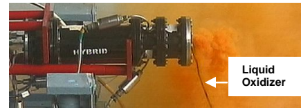
Fig.6. Test-02 of HTPB with 10%AP and RFNA
