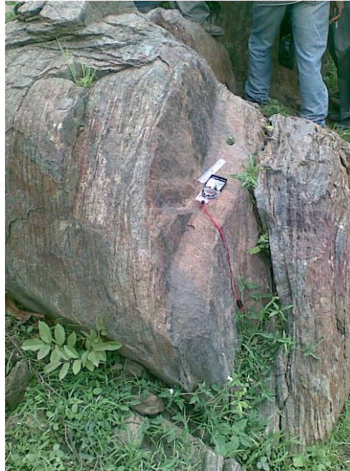
Fig. 9. Amphibolite schist outcropping beside college of arts & Islamic legal studies, Minna with 096^{\circ} strike & 78^{\circ} dip towards the north.
