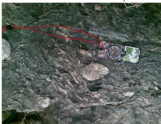
Fig. 10. Pebbly schist along Minna-Zungeru highway containing variably deformed clasts of granite, amphibolite schist, gneiss & quartzite. Strike is 160^{\circ} with 88^{\circ} NE dip.
