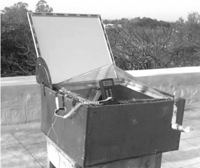
Fig. 2. Pyramid solar still with boosting mirror.
