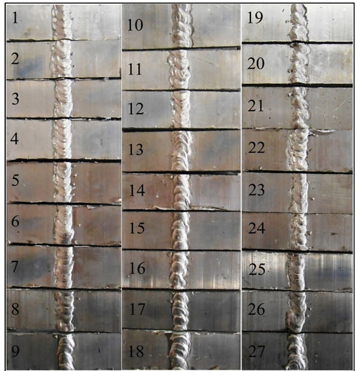
Fig.11. Penetration vs. welding current for 50 cm/min welding speed.
