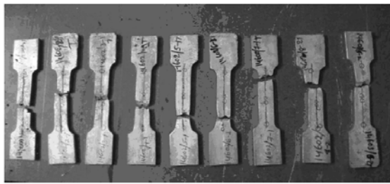
Fig. 3. Tested tensile Al/SiC composite specimens
