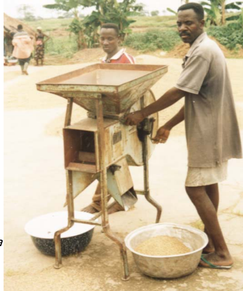
Fig. 2. Manual winnowing-machine in Togo
